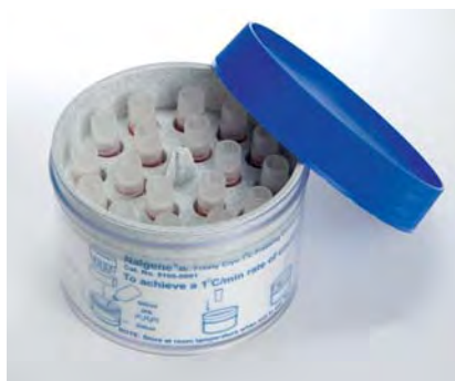
Mr. Frosty insert keeps tubes from contacting alcohol
